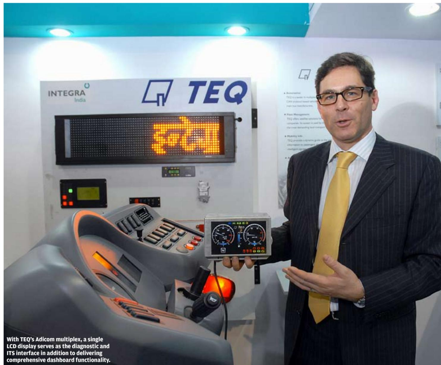
With TEQ's Adicom multiplex, a single LCD display serves as the diagnostic and ITS interface in addition to delivering comprehensive dashboard functionality.
